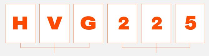
Product Platform High Voltage Generator Max Output Voltage E.g. 225kV
